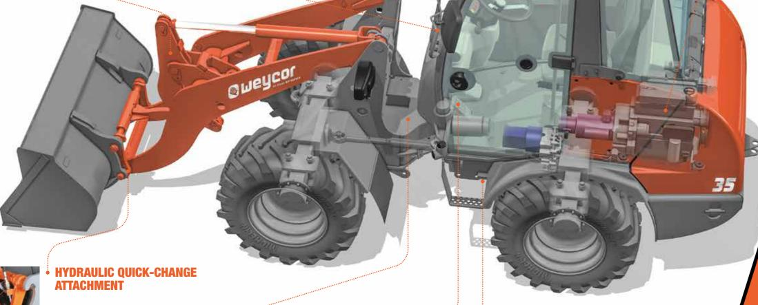
By allowing you to change the wheel loader's attachments in a few seconds, it turns the vehicle into an all-rounder.
