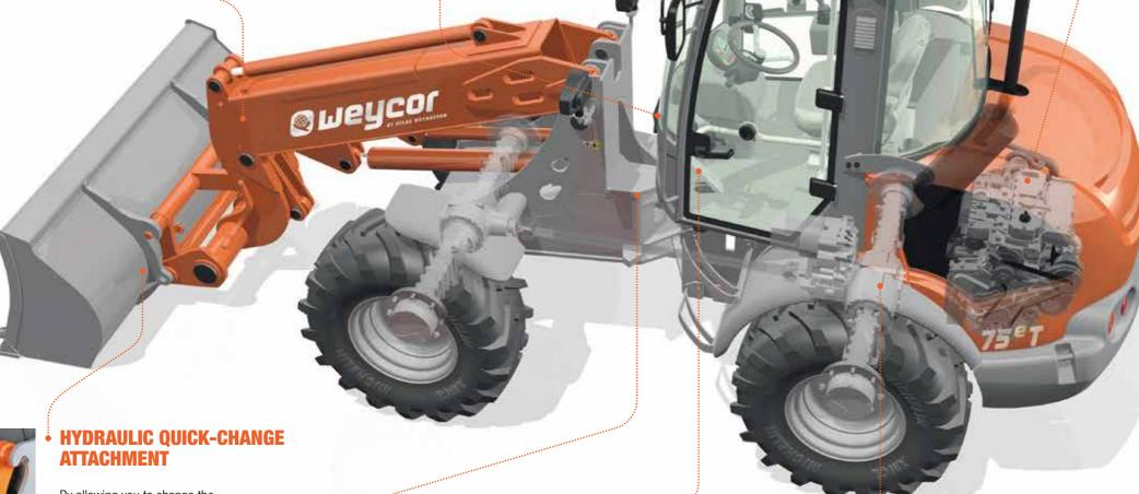
By allowing you to change the wheel loader's attachments in a few seconds, it turns the vehicle into an all-rounder.
